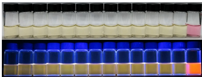
Figure 4. Photograph of 1 ( 10^{-5} M in MeOH) showing the color change (upper) and emission enhancement at 365 nm (UV lamp) (down) in the presence of various metal ions (2 equiv). From left to right: blank, \text{Cu}^{2+} , \text{Zn}^{2+} , \text{Pb}^{2+} , \text{Na}^+ , \text{Ni}^{2+} , \text{Co}^{2+} , \text{Cd}^{2+} , \text{Ba}^{2+} , \text{Mg}^{2+} , \text{Li}^+ , \text{Fe}^{2+} , \text{Ag}^+ , \text{Hg}^{2+} .
