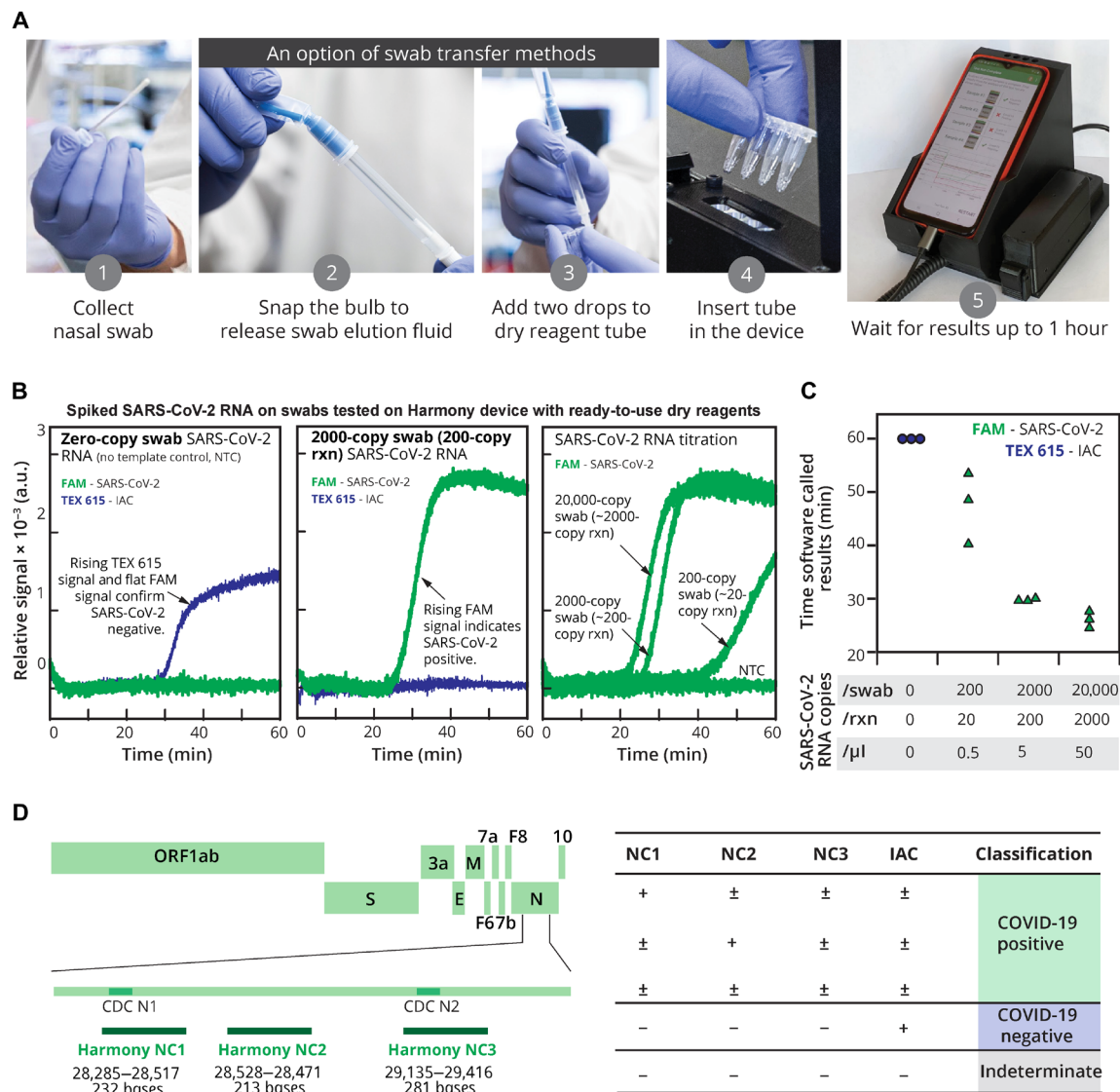
Fig. 1. Harmony COVID-19 workflow, analytical performance, and interpretation. (A) User workflow. A nasal swab is collected and eluted in the rehydration buffer using either a unified sampler dispenser (shown) or a tube-and-bulb method (Fig. 8). The swab eluate is then transferred into the reaction tube to rehydrate lyophilized and preloaded RT-LAMP reagents. Users follow the instructions on the cell phone app to record the sample identity, insert the tube in the test slot, and close the device. Four samples can be analyzed in parallel. Photo credits: (1) to (4), Mark Stone at the University of Washington; and (5), Christopher Snyder at North Seattle College. (B) Examples of on-device analysis. Lyophilized reagents were rehydrated with the eluate from swabs spiked with 0, 200, 2000, or 20,000 copies of SARS-CoV-2 RNA, run on the device, and analyzed in real time. The samples with SARS-CoV-2 RNA at 2000, 200, and 20 copies per reaction (rxn) were reported as positive by software at 27, 30, and 41 min, respectively; after 60 min, the NTC reaction was classified as negative. a.u., arbitrary units. (C) Time to result. Individual detection time points ( n = 3 ) are plotted. Variation in detection time increases as samples approach the detection limit. (D) Diagnostic algorithm. Harmony COVID-19 software calls samples as positive, negative, or indeterminate (IND) based on detection of the three regions in the nucleocapsid gene [Harmony NC1 overlapping with the CDC N1 region, Harmony NC2 (overlapping with CDC N3 region excluded from the current kit), and Harmony NC3 overlapping with the CDC N2 region] and the engineered IAC sequence.
