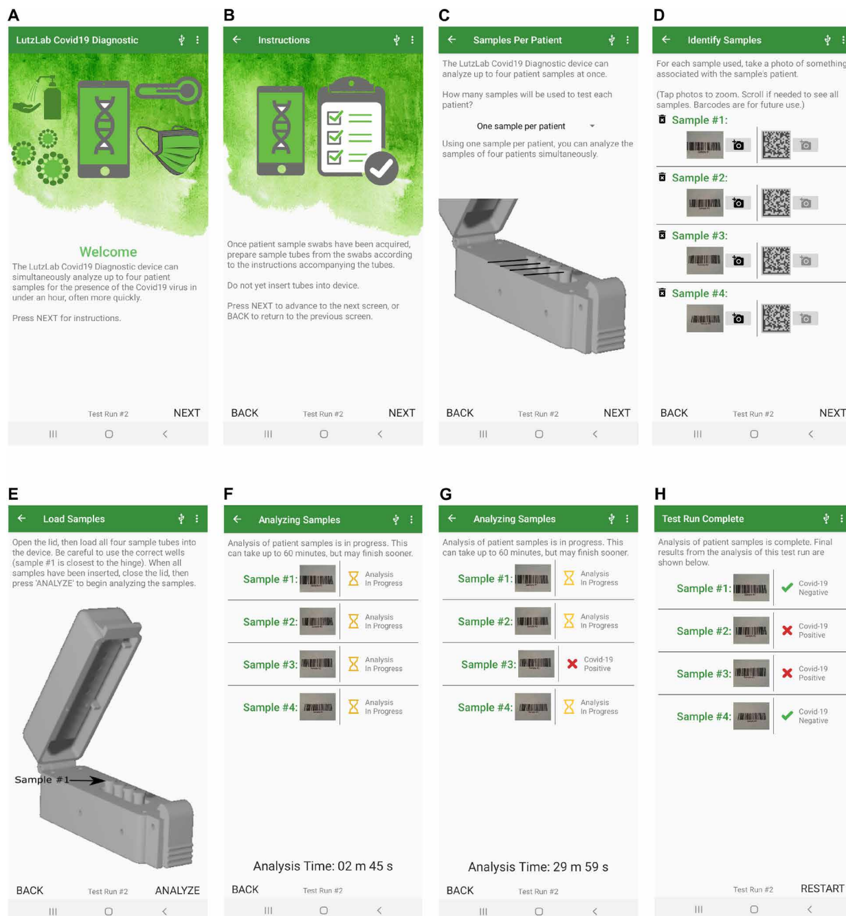
Fig. 5. Cell phone user interface and result reporting. The Android Harmony application guides the user through steps to set up and run the test. (A) Intended use of the device. (B) Instructions for the user to prepare samples. (C) Selection of the number of samples. (D) Collection of sample identifiers by barcode, photo capture, or manual typing. (E) Instruction to insert the tube when the temperature of the device reaches the reaction temperature. (F) Real-time analysis during the test run. (G) Positive results are reported as soon as they are detected. (H) Negative and IND results are reported at the end of the run time.
