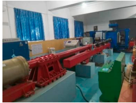
Figure 2. Triaxial static-dynamic comprehensive loading test system.
