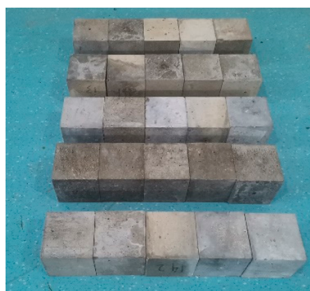
Figure 1. Concrete specimens eroded at different times.
