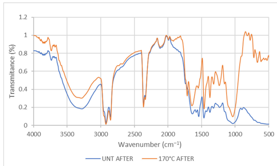
Figure 3. Comparison of IR spectra between EFB untreated and treated with 170 °C samples after wetting with oil. UNT: Untreated.
