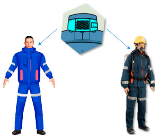
Figure 2. A view of protective clothing with PCM elements on the collar.
