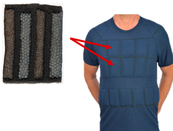
Figure 1. A view of protective T-shirt with PCM elements.
