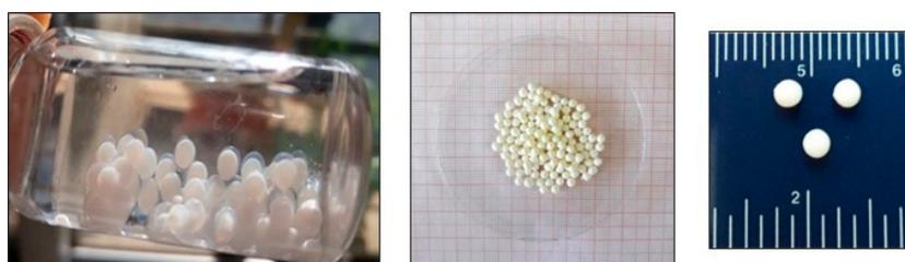
Figure 9. Photographs of PUA aerogel beads (wet-gels and aerogels) [94].
