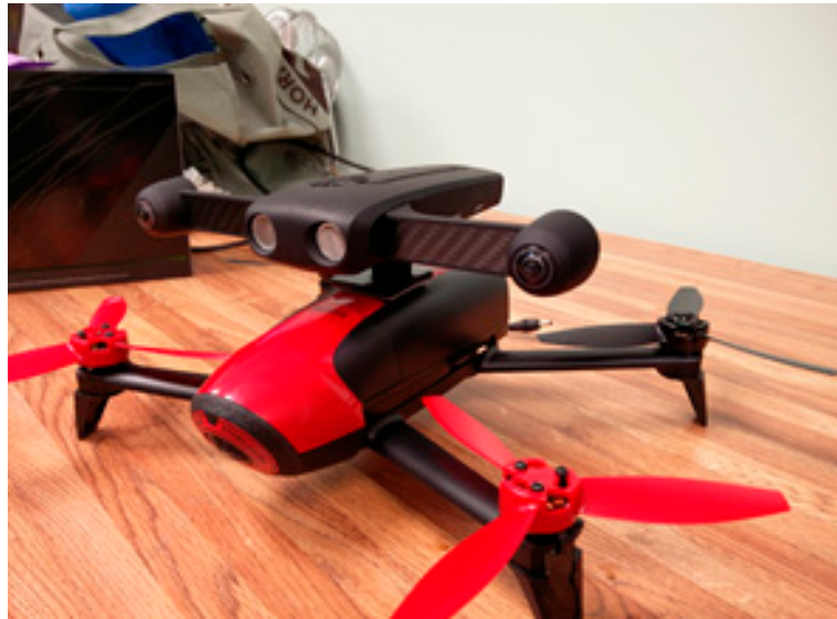
Figure 8. The testing hardware setup—A SLAM dunk mounted on a Parrot Bebop 2 drone.
