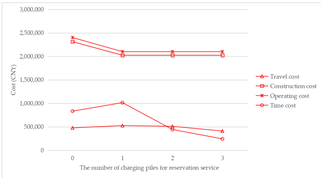
Figure 10. Cost change with a changing number of charging piles for the reservation service under \tau = 0.2 .
