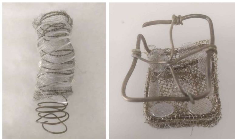
Figure 2. Polymer metal supports used over the impregnation process.
