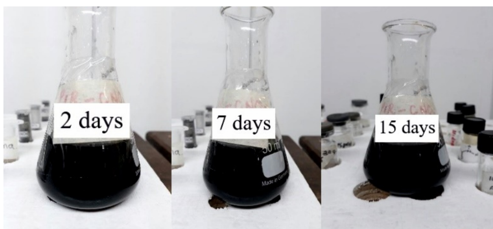
Figure 2. Dispersions of CNOs that were functionalized with the pyrene ( pyr -CNOs) in water.
