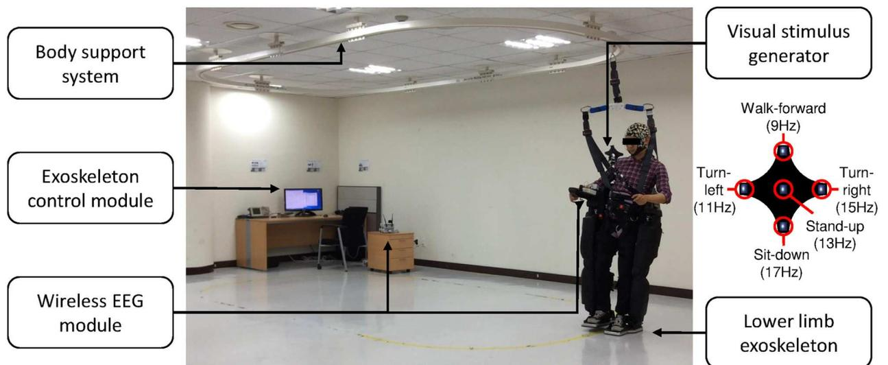
**Fig 1. Experimental environment.** Subject wearing the lower-limb exoskeleton and focusing on an LED from the visual stimulus generator. The EEG is transferred by a wireless interface to the PC. A body support system (a rail beneath the ceiling) was connected to the subject for safety purposes. The exoskeleton was controlled by an external operator using a keyboard controller.
