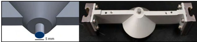
FIGURE 2. The surface area of the pin tip of the upper platform of the SimpleCAT was precision engineered to produce an even pressure distribution on the tissue with minimal areas of stress concentration.
