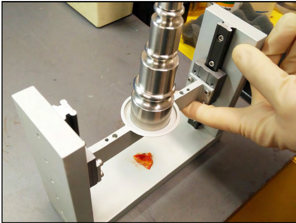
FIGURE 3. Weights are first loaded on to the platform and then the platform lowered onto the tissue to induce compressive stress.
