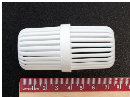
FIGURE 1: Plastic cage used in the dissolution experiments to avoid eventual adhesion to the vessel or floating.
