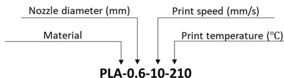
**Fig. 2.** Naming samples based on the parameters used for printing.
