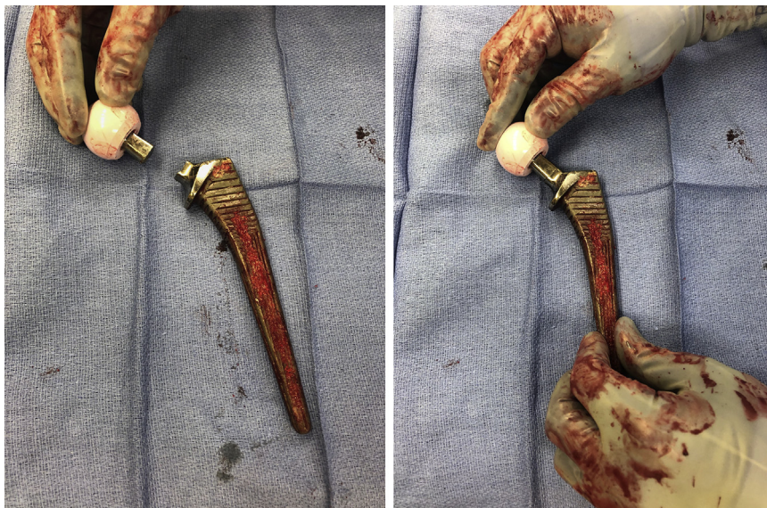
Figure 3. Intraoperative pictures of the broken stem. The midportion of the neck is broken with a transverse pattern.
