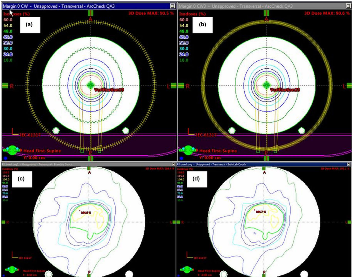
FIG. 6. Differences in isodose distributions between the distributed calculation framework (DCF) angular resolution settings (a) 5 cm field, dynamic conformal arc with 5° DCF angular resolution setting (b) 5 cm field, dynamic conformal arc with 0.7° DCF angular resolution setting (c) Lung IMRT plan, DCF angular resolution setting of 5 degrees (d) Lung IMRT plan, DCF angular resolution setting OFF.
