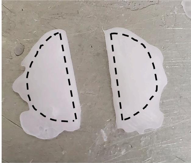
**Figure 6. ALI membrane halves embedded in paraffin wax**
