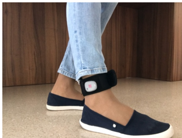
Figure 1. Dance motion capture. We use a single wearable device, including a micro-electromechanical system (MEMS) 3D accelerometer sensor, attached just above the dancer's right leg ankle. The microposition and orientation of the sensor are arbitrary.
