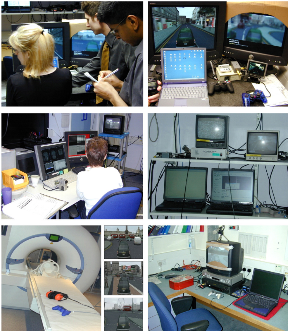
Fig. 1. The complex set-up used to run a virtual reality navigation fMRI study (Spiers and Maguire, 2006a — see text for details). This 'behind the scenes' view is rarely depicted in fMRI papers, and is in contrast to the experience of the participant (lower left) who uses a simple MRI-compatible games console, headphones and a screen to navigate in VR London. Snapshots of the simulation of London – middle bottom – are reproduced with the kind permission of Sony Computer Entertainment Europe.
