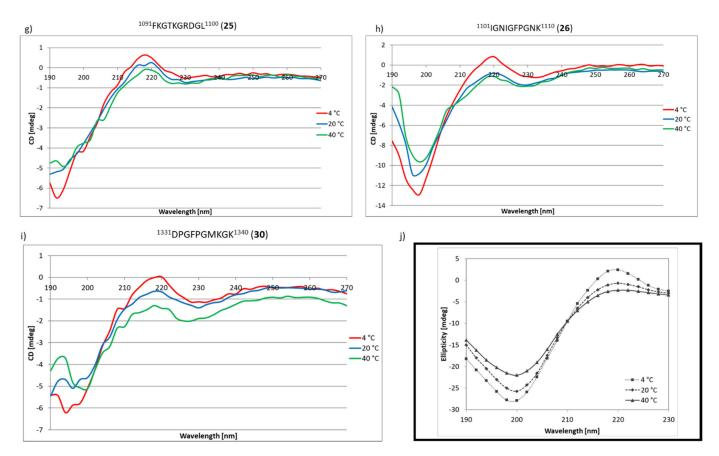
**Figure 9.** CD spectra of peptides: **2** (**a**), **4** (**b**), **5** (**c**), **6** (**d**), **14** (**e**), **15** (**f**), **25** (**g**), **26** (**h**), and **30** (**i**). (**j**) shows the CD simulated spectrum of the triple helix based on the literature data at different temperatures. The CD spectra were measured at 4 °C, 20 °C and 40 °C, after 24 h of incubation of the aqueous sample solutions at the same temperatures.
