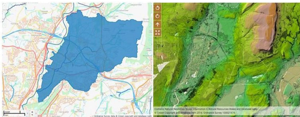
Figure 1. Map showing Nant-Y-Fendrod river catchment area (left) and LIDAR Digital Terrain Model showing topography of the study area (right). Contains Ordnance Survey Data© Crown copyright and database right 2013.
