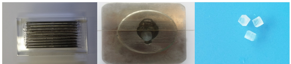
Fig 2. Porcine lens cutting methods. Left: Own cutting knife was made with acrylic plate and laser cutter with 2mm interval. Middle: The lens was trapped between the blades, cutting knife were inserted plate slots. Right: The porcine lens is cut into 2.0 mm 3 cubes.
