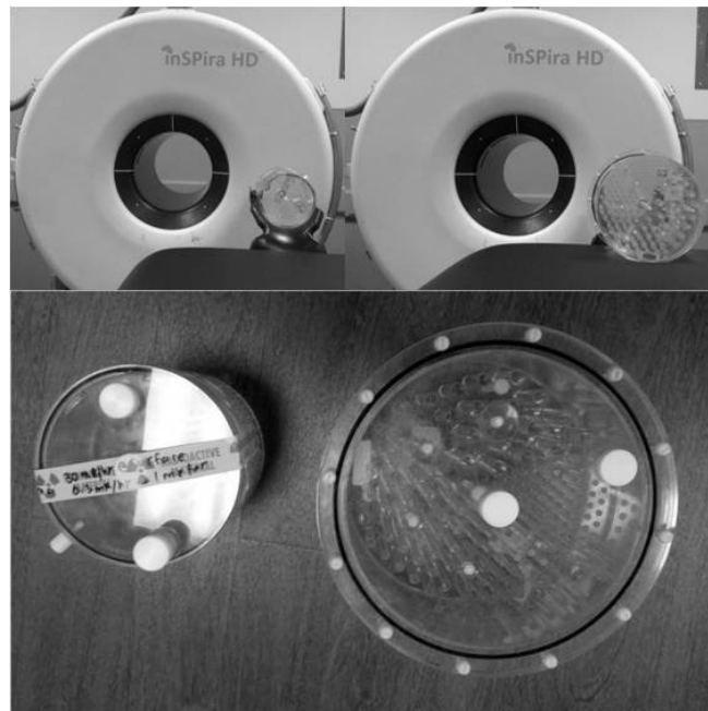
FIG. 2. Scanner bore and phantom. Top: Small (left) and flanged Deluxe (right) Phantoms next to SPECT scanner bore (note that the flanged Deluxe Phantom cannot fit in the head holder and cannot fit in the bore while resting on a platform). Bottom: Small (left) and flanged Deluxe (right) Phantoms.
