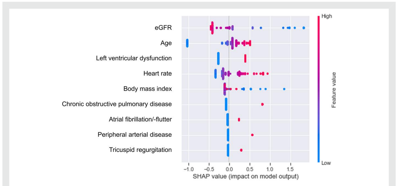
Figure 4 Shapley Additive exPlanations plot of feature importance in the final machine learning model. The importance of features is shown in increasing order on the y-axis (estimated glomerular filtration rate is the most important). The relative impact of these features on the model output is depicted on the x-axis (the right of 0.0 means increased risk and the left of 0.0 means reduced risk). The value of the feature is shown in colors. For example, a low estimated glomerular filtration rate is associated with a higher risk of mortality (on the right side of the x-axis), while a high estimated glomerular filtration rate (on the left side of the x-axis) has a protective effect. eGFR, estimated glomerular filtration rate; SHAP, Shapley Additive exPlanations.
