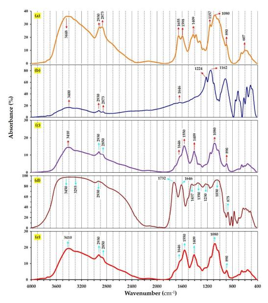
**Figure 4.** FT-IR spectra of (**a**) chitosan, (**b**) STPP, (**c**) empty CSNPs, (**d**) PPE and (**e**) PPE-loaded CSNPs (at chitosan: PPE ratio of 1:0.50 w/w).
