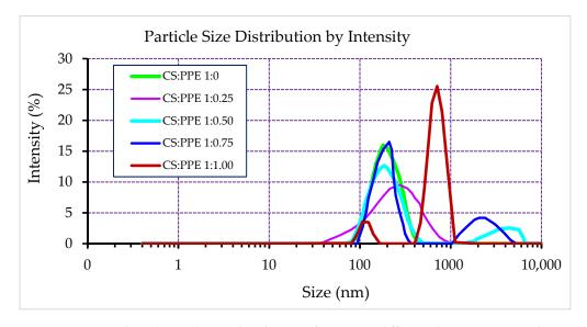
Figure 1. Intensity-based particle size distribution of CSNPs at different chitosan:PPE weight ratios.
