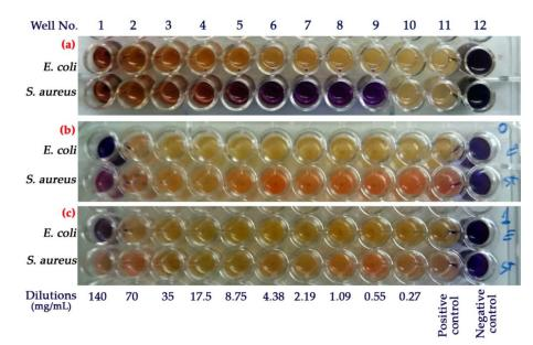
**Figure 6.** Results of antimicrobial test against *E. coli* and *S. aureus* using resazurin-aided microdilution method performed in 96-well microtiter plates. Samples: (**a**) PPE, (**b**) empty CSNPs, (**c**) PPE-loaded CSNPs (chitosan:PPE ratio of 1:5.00 w/w). Sample concentrations for well columns 1–10 are reported in the figure.
