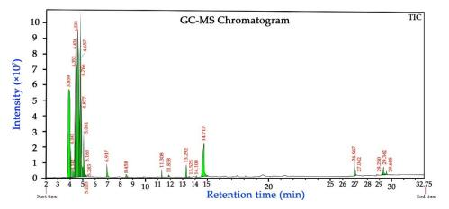
Figure 7. GC–MS chromatogram of methanolic extract of pomegranate peel.
