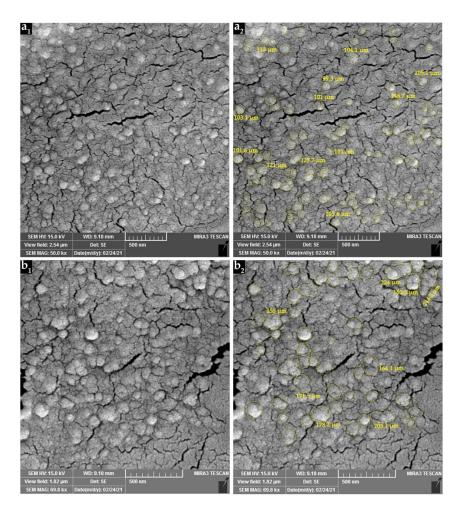
**Figure 3.** SEM image of  $(a_1)$  empty CSNPs, and  $(b_1)$  PPE-loaded CSNPs at chitosan:PPE ratio of 1:0.50 (w/w). Images  $(a_2,b_2)$  represent processed figures using ImageJ.
