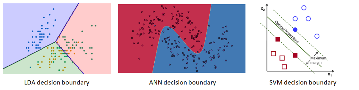
Figure 2. Decision boundaries for the different classifiers (Linear Discriminant analysis (LDA), Support Vector Machines (SVM), and Artificial Neural Networks (ANN)).
