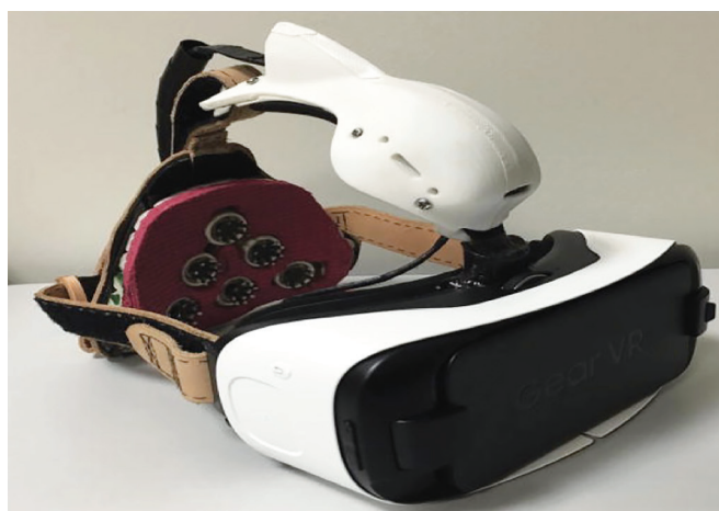
Fig. 5: Portable brain-computer interface for objective assessment of visual function loss (Nakashini et al.)
