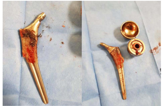
Figure 3. Intra-op pictures of the prosthesis, showing the bend at the neck-taper junction.
