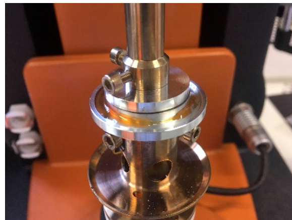
Figure 7. Shear rheology sample preparation showing the excess material and 0.6 mm gap.
