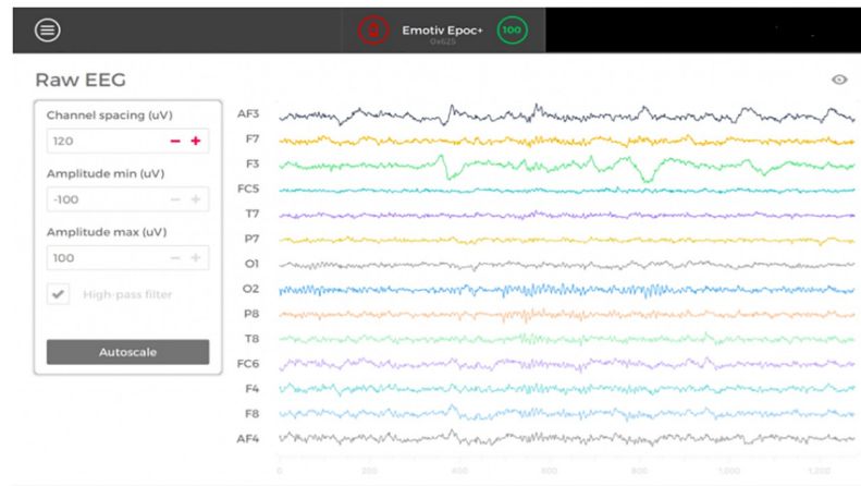
Fig 3. Raw EEG data obtained from the 14 channels of the Emotiv EPOC headset.
