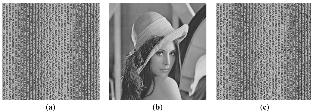
Figure 8. (a) The array transformed from the secret text with m = 2 . (b) The image embedded with hidden data with \alpha = 0.05 . (c) The recovered transformed array. The recovery accuracy is 100%.
