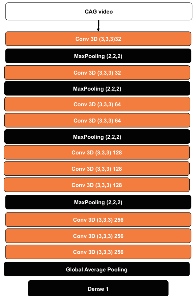
Fig. 1. Structure of the neural network and input data for the model
