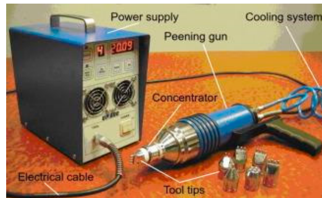
Figure 5. Ultrasonic peening equipment. Reproduced with permission from [80]. Copyright Elsevier, 2015.
