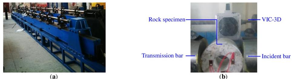
**Fig 1. Mechanical test system with radial impact of circular granite specimens. (a) SHPB and (b) VIC-3D.**
