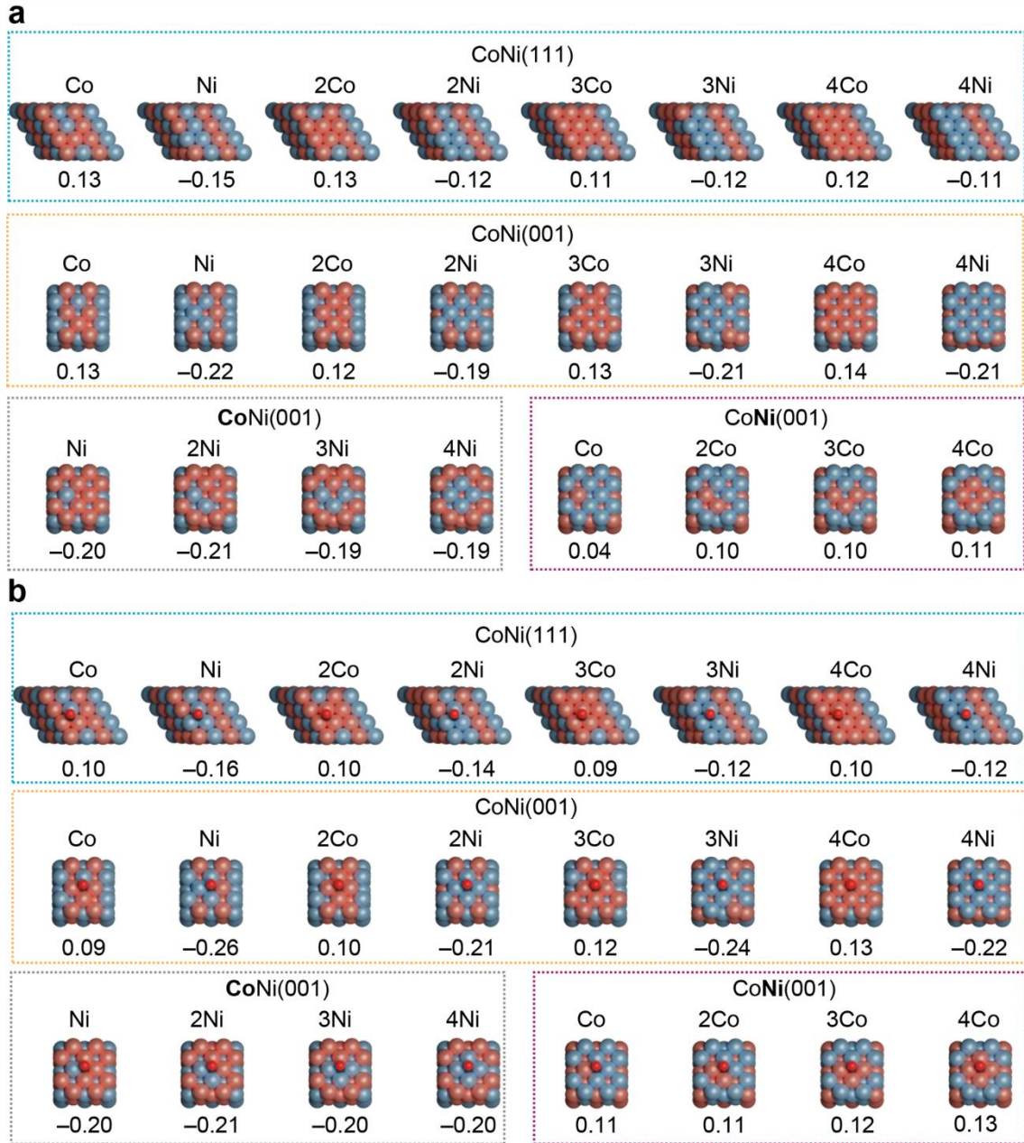
Supplementary Fig. 33 | DFT models employed to evaluate the segregation energy ( E_{\text{seg}} , eV/segregated atoms) for various Co-Ni alloy models with and without adsorbed CO. a , Snapshots of bare Co-Ni alloys featuring different numbers of Co/Ni segregated atoms and their corresponding E_{\text{seg}} values. b , Snapshots of Co-Ni alloys with adsorbed CO, featuring different numbers of Co/Ni segregated atoms and their corresponding E_{\text{seg}} values. The alloys models were framed with dotted lines in different colors, corresponding to the colors of the markers in the plots of Supplementary Fig. 32. Color code: Ni (blue), Co (light pink), C (dark gray), and O (red).
