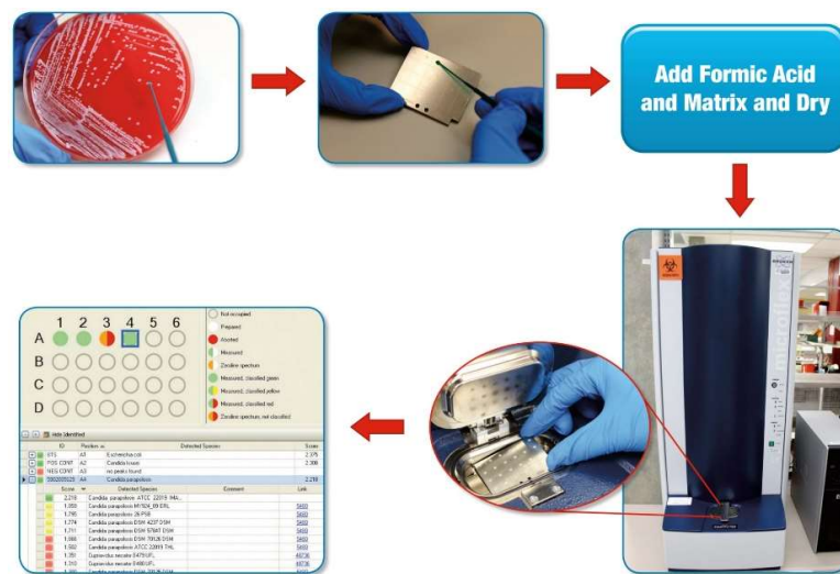
Figure 1. Process of matrix-assisted laser desorption ionization time-of-flight mass spectrometry (MALDI-ToF MS) for yeast identification [7,8]. A colony is picked from a culture plate to a spot on a MALDI-ToF MS target plate (a disposable or reusable plate with a number of spots, each of which may be used to test different colonies). For yeast applications, cells are typically treated with formic acid on the target plate, followed by drying. The spot is overlain with 1–2 µL of matrix and dried. The plate is placed in the ionization chamber of the mass spectrometer (Figure 2). A mass spectrum is produced and compared against a library of mass spectra by the software, resulting in identification of the yeast ( Candida parapsilosis in position A4 in the example). Used with permission of the Mayo Foundation for Medical Education and Research. All rights reserved.
