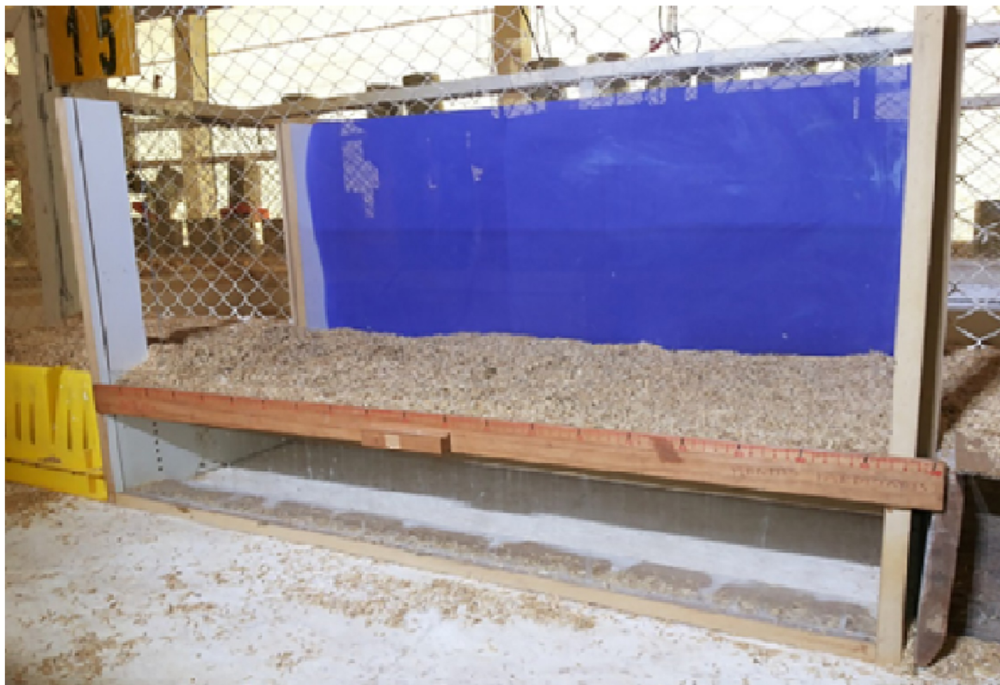
Fig 1. Test area 1 m x 30 cm, flat surface, and 8 cm deep aviary bedding (wood shavings), 50 cm tall acrylic plates were placed at the sides of the track.
