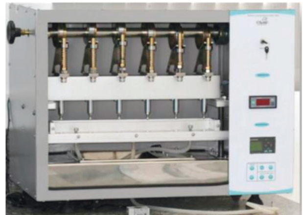
FIGURE 3: Electromechanical mastication fatigue testing equipment.
