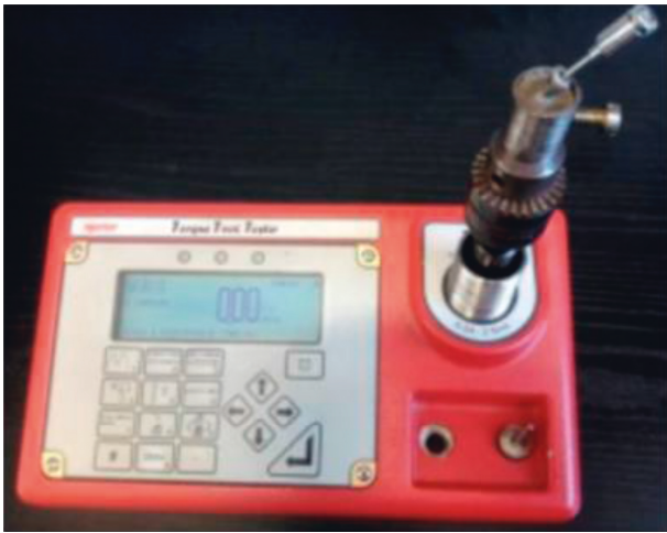
FIGURE 2: Digital torque gauge (torque tool tester, TST série 2 Norbar®, Navi Mumbai, India).
