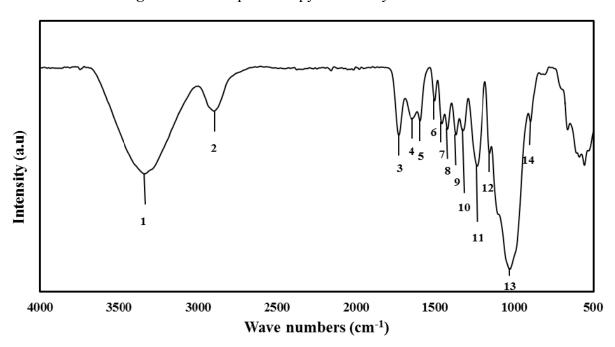
Figure 2. FT-IR spectroscopy of undecayed rubberwood.
