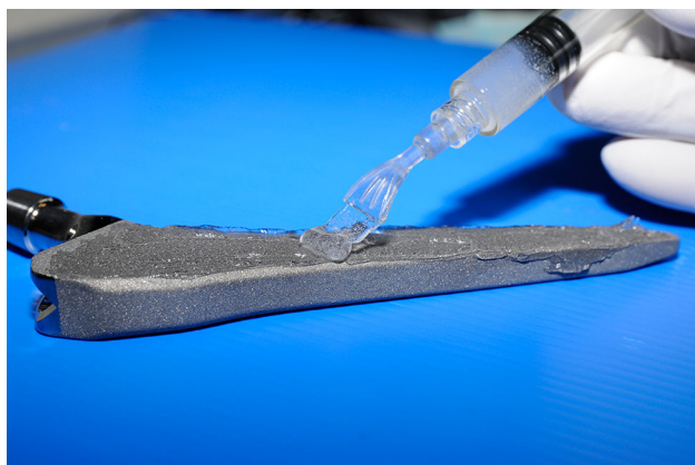
Fig. 1 Spreading of the hydrogel on a titanium prosthesis through a suitable syringe spreader is shown.
