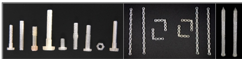
Figure 4. FDM 3D-printed orthopedic screws, plates and pins of PLA. Reprinted from Tappa et al. [35], licensed under CC BY 4.0.
