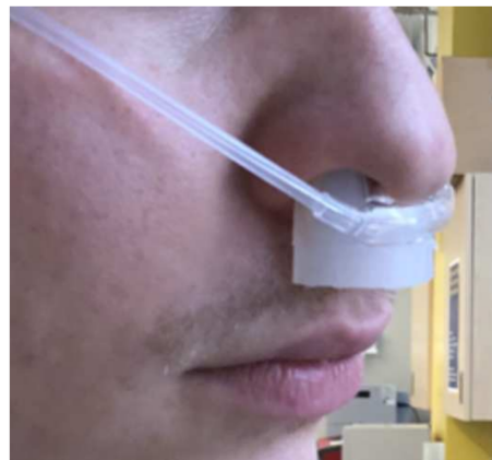
Figure 2. This figure shows the placement of the nasal septum sensor in an imaged nose, indicating the positioning of the device within the nasal cannula. This placement was modeled on a team member.
