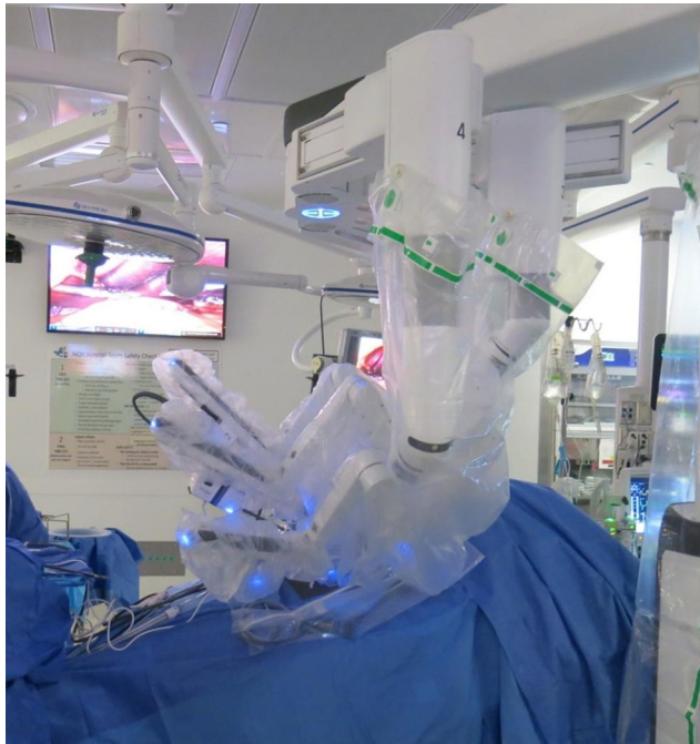
Figure 3 Intraoperative photograph with the robotic surgery system docked at the operating room table which is in reverse Trendelenburg position to facilitate surgical visualization of the abdominal contents. The patient's head is to the right.
