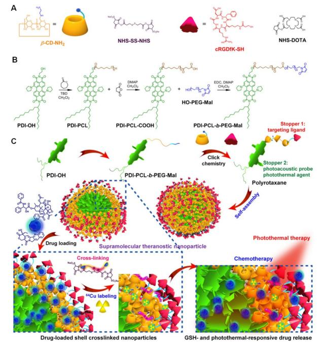
Figure 4. Synthesis and fabrication schematics of SCNPs for supramolecular theranostics. (a) Chemical structures and cartoon representations of the building blocks. (b) Synthetic route to the polyrotaxane. (c) Schematic illustrations of the preparation of drug-loaded SCNPs and dual-responsive drug release. Reproduced with permission from [104], copyright 2018 Nature Publishing Group.
