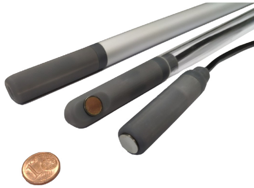
Fig. 2. Thermal Endoscope System prototypes assembled, for frontal and lateral vision.
