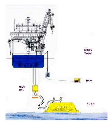
**Figure 3.** Works on an oil rig. The divers are supplied from a diving bell that in turn is supplied by a diver support vessel (see Figure 2). The divers are surveyed by a remotely-operated vehicle (ROV). Reprinted with permission from [5]. Copyright 2012 slideshare.net.
