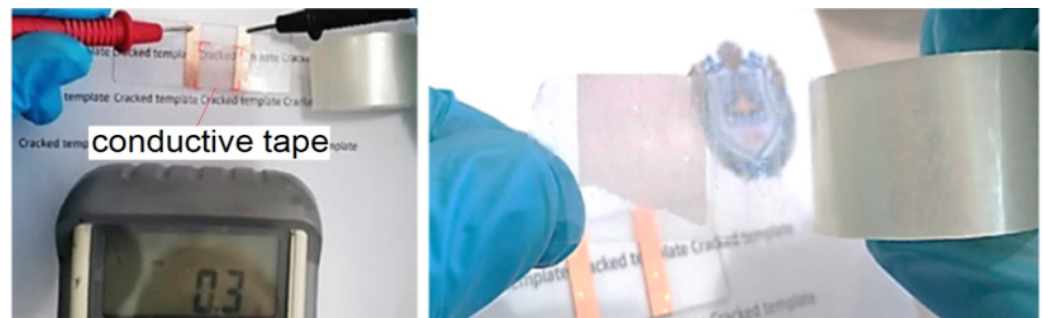
Figure 10. Example of obtaining electrically conductive scotch tape based on SCM 180.
