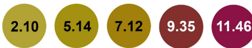
Figure 4. Colors of the curcumin-cellophane sensors after exposure to standard pH solutions (Radelkis Kft., Budapest, Hungary; pH 2.10, 5.14, 7.12, 9.35, and 11.46 ( \pm 0.03 at 25 °C)) [75].
