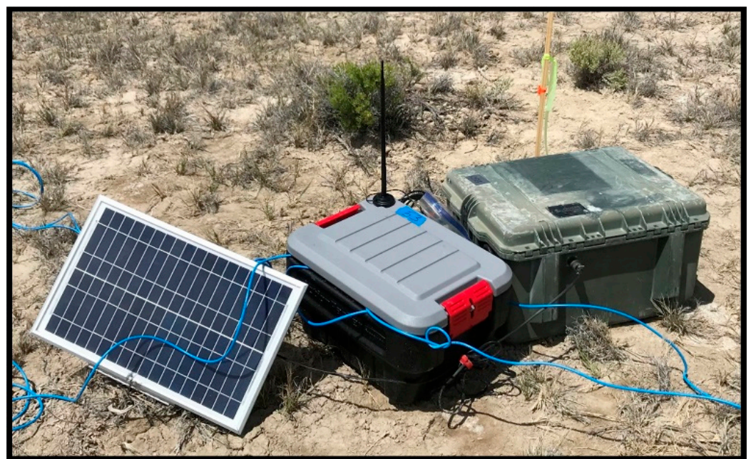
Figure 10. San Emidio Geothermal Field T&E event lower layer edge device and edge gateway.
