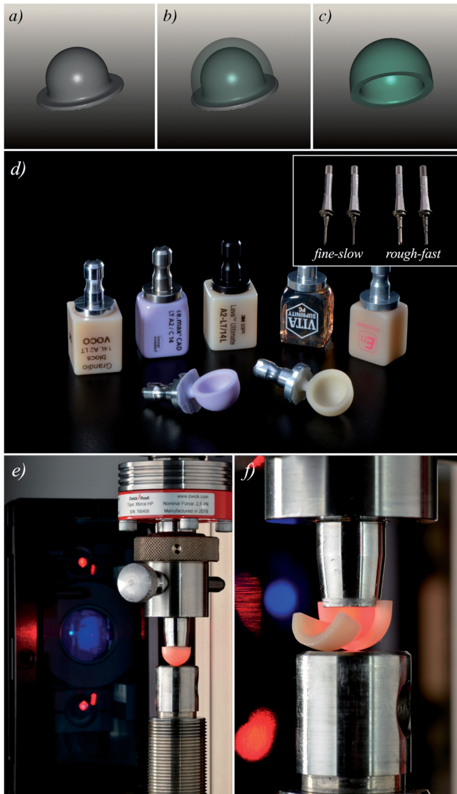
Figure 1. (a) Scanned abutment, (b,c) designed spherocylindrical shape to be machined, (d) CAD/CAM materials investigated in this study before and after machining (inset shows the burs used in the two different machining protocols), (e) marginal strength test is performed with a laser extensometer, and (f) a view of a fractured specimen [Reprinted with permission from Elsevier].
